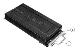
PRESS are available: for 8 exposures of  $6\times9$  cm negative size from a roll of 120 film, or for 10 exposures of  $6\times7$  cm negative size. Both holders can be used for taking pictures of  $6\times6$  cm or  $6\times4.5$  cm size; however filmwind stop and exposure counter cannot be used in this case, the red window must be used for visual check of film advance.
